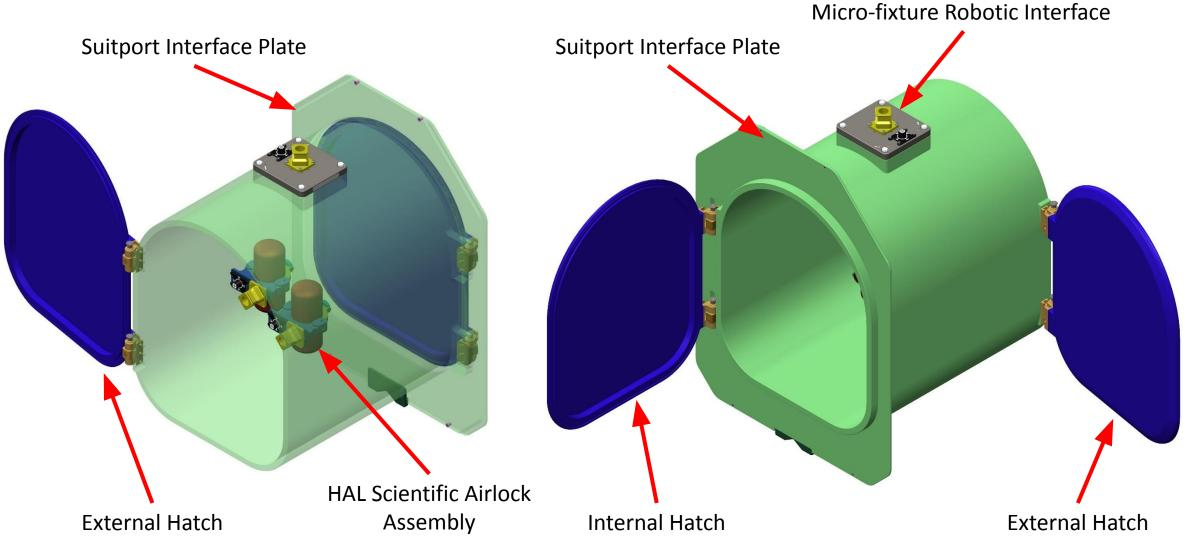
Note: HAL Scientific Airlock Suitport Interface Plate (SIP) and hatches are based on suit port rear entry hatch. External hatch is electrically driven.
