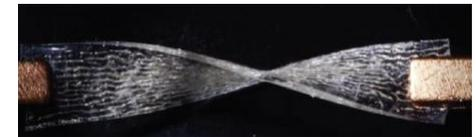
Ag-coated fiber elastomeric composite
