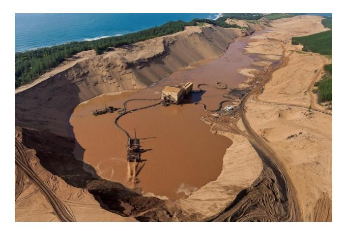
The current process consists of dredging and physically separating the valuable heavy minerals sand from silica sand using centrifugal spirals and electrostatic and magnetic separators (Average ratio of 5-10% HM to 90-95% silica). The process does not require chemical processing of the minerals. On average, Rio Tinto mineral sand dredging operations are mining approximately 100 to 200 Hectares of land yearly.
