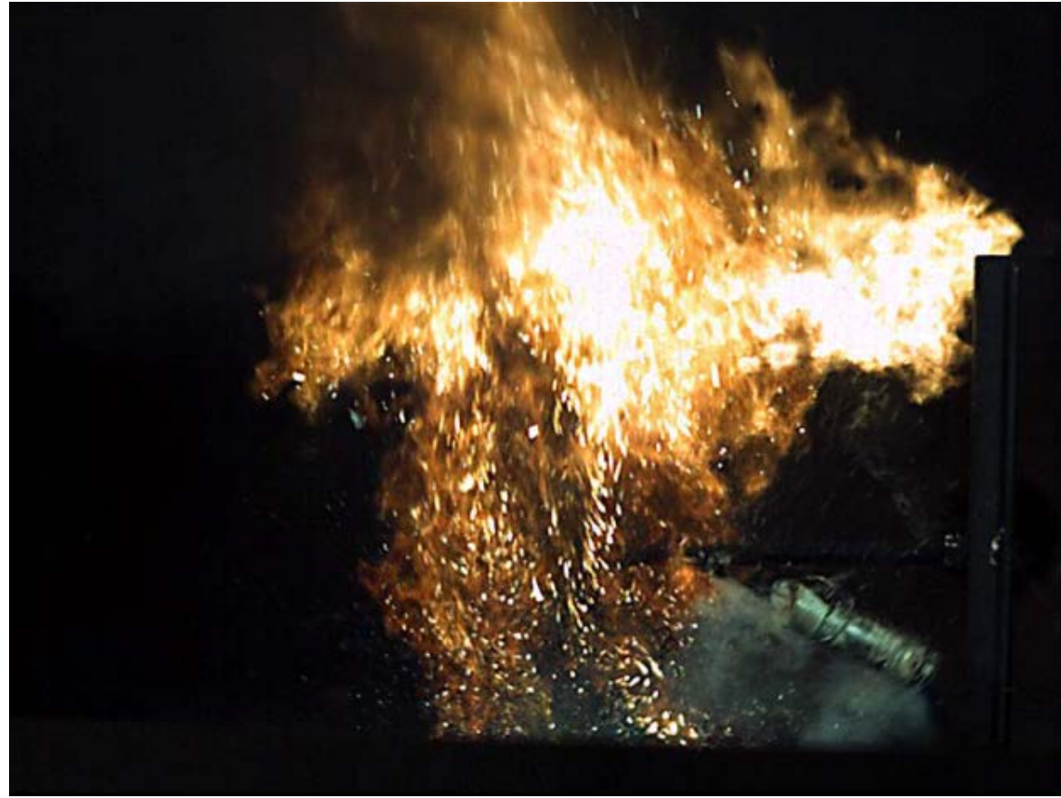
LiCoO 2 cell in catastrophic disassembly
