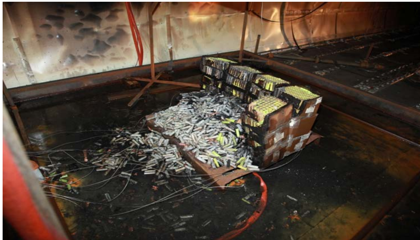
LiCoO 2 cell in catastrophic disassembly
