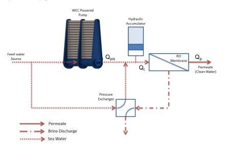
Figure 1. Schematic representation of the wave-powered reverse-osmosis (RO) desalination system.
