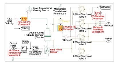
(b) Hydraulic cylinder and direction valves
