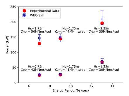
Figure 4. Comparison of power performance from WEC-Sim (using a linear damper) and van't Hoff's experimental measurements (presented in full scale).
