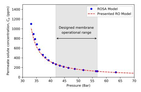
Figure 6. Influence of feed pressure on the water quality (salinity) of the permeate flow.
