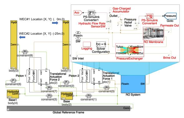
Figure 11. WEC-Sim model for the two-WECs-coupled desalination system.
