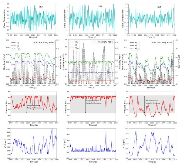
**Figure 10.** Time history of wave elevation and the dynamics of the RO desalination system (row 1: SS2; row 2: SS3; row 3: SS4; col 1: wave elevation; col 2: flow rate & recovery ratio; col 3: pressure; col 4: permeate solute concentration.
