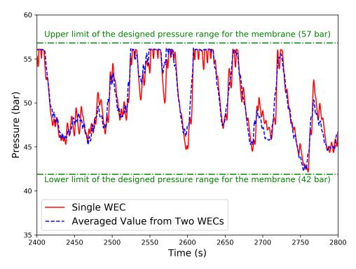
**Figure 12.** Hydraulic pressure time history from the WPDS and the averaged value from the two-WECs-coupled WPDS case.
