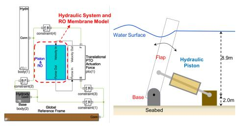
Figure 2. WEC-Sim wave to water model (left) and schematic representation of the OSWEC (right).
