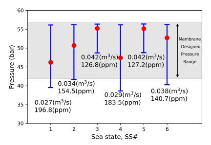
Figure 9. Summary of the WPDS overall efficiency under different wave conditions.
