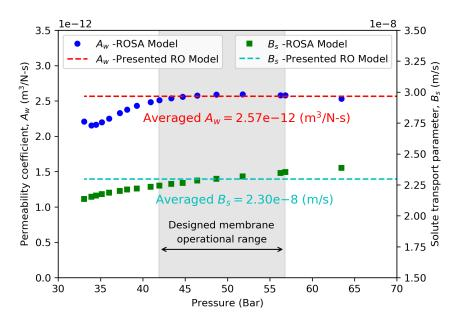
Figure 5. Influence of feed pressure on the permeability coefficient and solute transport parameter.
