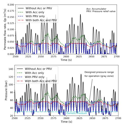
Figure 7. Time history of the permeate flow rate (top) and pressure (bottom) for SS2.
