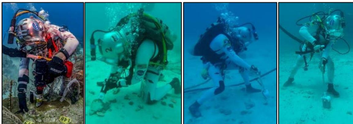
**FIGURE G-2: POWERED AND MANUAL EVA SAMPLE ACQUISITION TOOL CONCEPTS (CORE, CHIP, SOIL, SURFACE)**
