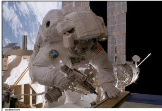
**FIGURE G-1: UTILIZING THE PISTOL GRIP TOOL (PGT) DURING AN ISS EVA**
