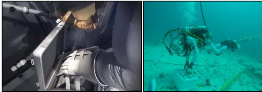
**FIGURE 6.1.3-3: ASTEROID SAMPLE STOWAGE CONCEPT (ARMC) AND EVALUATIONS DURING NEEMO 20**
