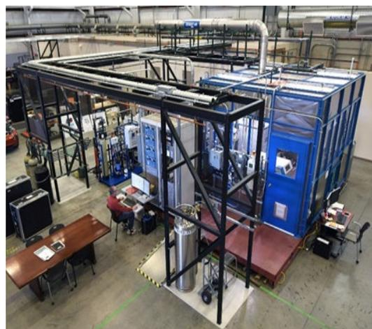
Overview of the 25-kW HTSE experiment skid and enclosure within the INL System Integration Laboratory.
