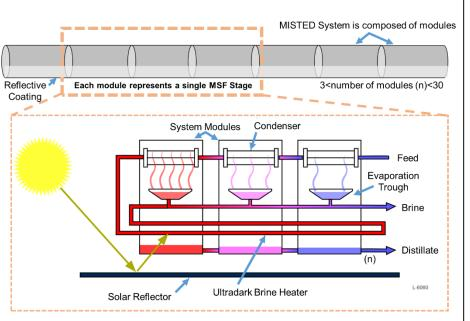
Modular MISTED system stacks layers of multi-stage flash (MSF) for highly scalable design
