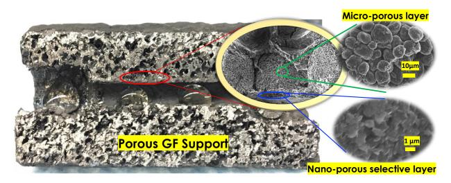
Figure 1. Superhydrophobic coated graphite foam tubular membrane.
