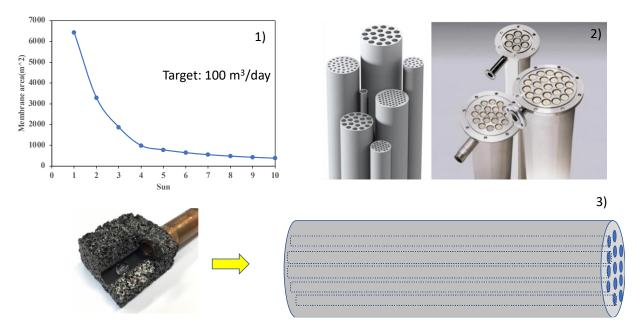
**Figure 2** 1) Solar Membrane area requirement as a function of solar intensity; 2) A commercial multi-channel inorganic membrane and module to pursue in MIST devices; 3) Proposed multi-channel GF membrane.
