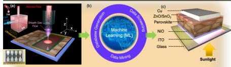
Schematic of (a) thin-film deposition of perovskite by an aerosol-jet assisted spray coating (AJSC) process (inset: fabricated perovskite solar cells on glass), (b) development of machine learning for process optimization, and (c) targeted low-cost perovskite device structure to be studied in this project.
