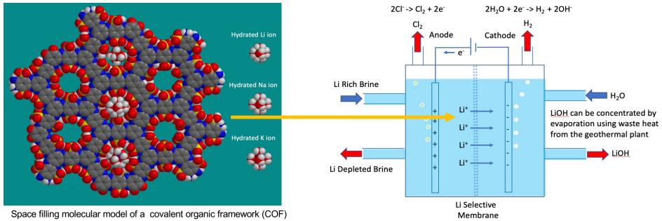
Space filling molecular model of a covalent organic framework (COF) membrane showing how the highly negatively charged pores with six sulfonate groups that strongly attracts cations is just the right size to allow lithium ions to go through while sodium and potassium ions are too large to pass.
