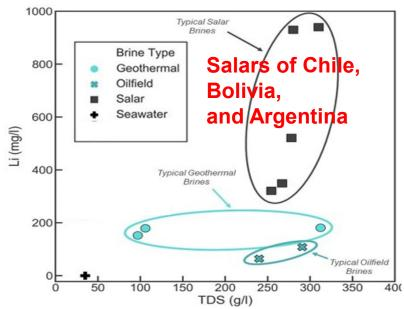
Geothermal brine is harder to extract due to lower Li<sup>+</sup> concentration and presence of other background ions.
