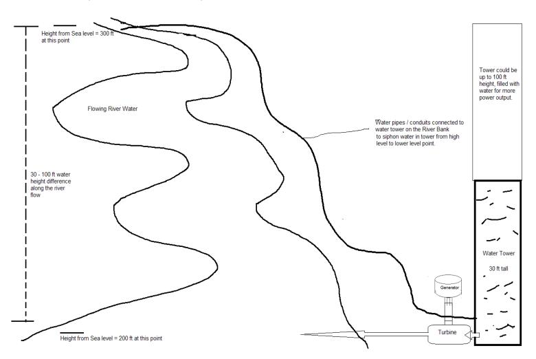
We can siphon the water from high level to lower level easily using multiple pipes / conduits. When they all are connected to a water tower, very high amount of input flow is generated. Water continuously flows in tower and is released at the bottom and fed to turbine, which generates power. Multiple turbines can be operated on single water tower or they can be distributed along the river side at suitable sites / distances.
