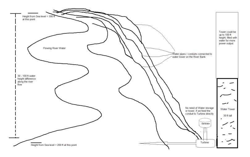
As an example, let's consider one conduit carries 1000 gallon water per min into the water tower. If we have 10 conduits, we will be filling the tower at 10000 gallon per min. If we have bigger conduits, we can carry high amount of water into the water tower. In this way 1000000 gallons of water enters in Water tower and leaves from the bottom to turbine making as much energy as a Dam Hydro plant can make.
