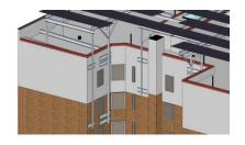
Exterior-wall-attached structural straps minimize load on roof and allow for spans of up to 40 feet
