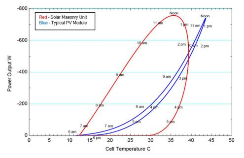
Modules bonded to thermal mass run up to 10 °C cooler and can recover up to 5% of the power lost to overheating from the sun.
