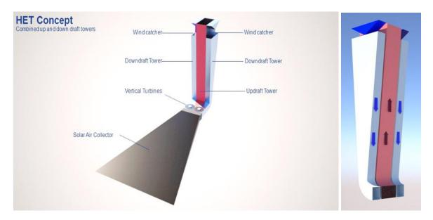
The Solar Thermal Power Tower includes transpired solar air collectors, solar updraft tower, wind downdraft tower, Venturi or diffuser chamber for turbines, phase change material (PCM) thermal storage and integration of PV with recovery of wasted PV heat.
