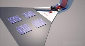
Heat from transpired collectors provide the driving force and can be coupled with PV arrays in a PVT configuration to recover the thermal energy and produce more power.
