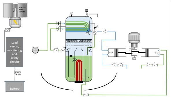
This proposal is a primarily solar thermal heated, small scale, low pressure vapor distillation unit. It is of a metallic shell construction where internal and external flowpaths are deliberate in efficient regenerative heat exchanging processes. This unit is designed for coastal areas to take advantage of solar and wind resources. The primary use for this unit would be desalination of ocean salt water for potable purposes.
