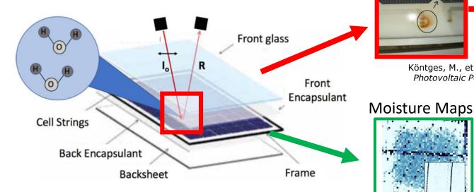
PV WaRD is a **non-destructive** optical method to detect **moisture** that can be used to forecast deterioration basedon the water content and quality of your modules.
