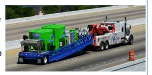
Our solution is a portable, unitary, non-biological sewage treatment and water reclamation system adapted to be moved without disassembly on national and state highways between temporary sites, and capable of processing any volume/flow rate of biologically charged wastewater to drinking water standard in under 24 hours.
