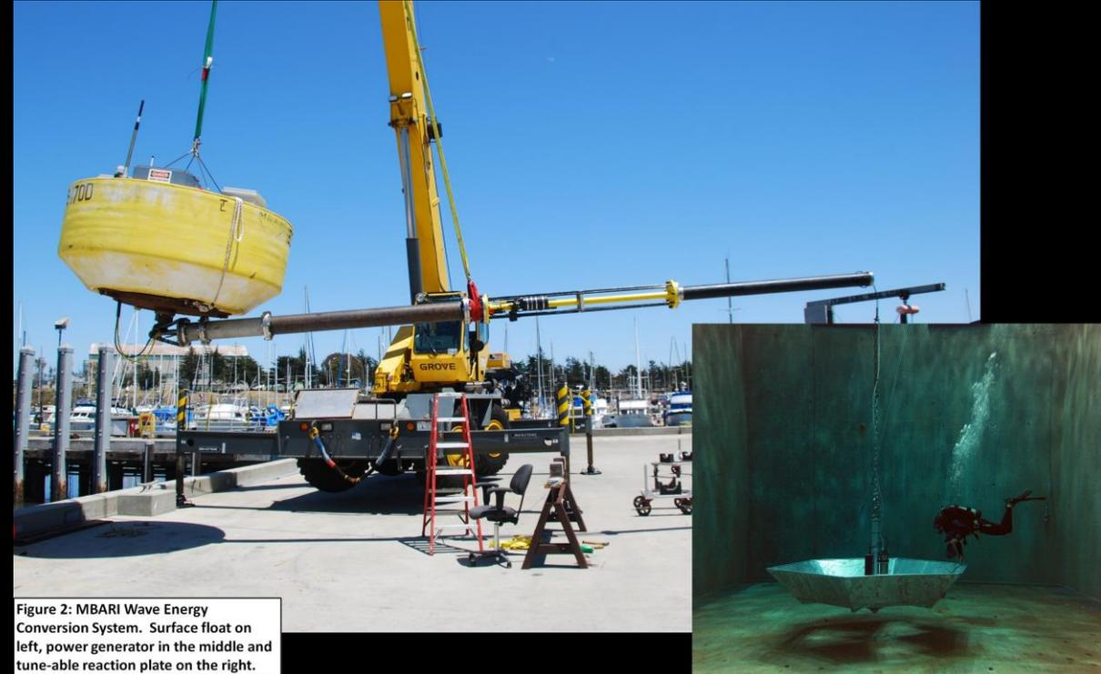
Figure 2: MBARI Wave Energy Conversion System. Surface float on left, power generator in the middle and tune-able reaction plate on the right.
