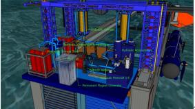
ft. pound hydraulic motors then to 10 mw permanent magnet generator-then to the electrolysis machine that generates hydrogen then stores it in the red tanks. A fuel cell is included to provide electricity for shipboard operations and fuel for the ship.
