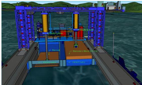
The primary impound area leads to the sub impound area that houses the 100-ton weighted buoyancy blocks. They are connected to large Hydraulic cylinders. A series of wicket gates controls the flow of seawater in and out of the areas causing the block rises and falls with the entry seawater. The weight of the block pressurizes the hydraulic fluid to 2000 psi
