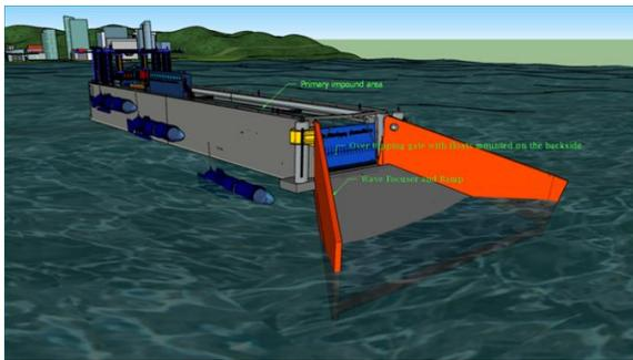
The over-topping gate prevents seawater from draining out.
