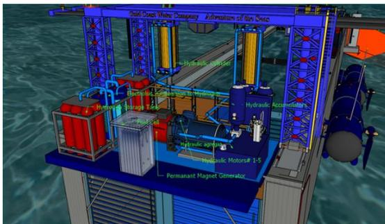
The pressurized seawater then goes to accumulators then into 2 million ft. pound hydraulic motors then to 10 mw permanent magnet generator-then to the electrolysis machine that generates hydrogen then stores it in the red tanks. A fuel cell is included to provide electricity for shipboard operations and fuel for the ship.
