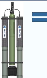
2 Seatrec SL1 thermal energy harvesting modules attached to Sea-Bird Scientific Navis float
