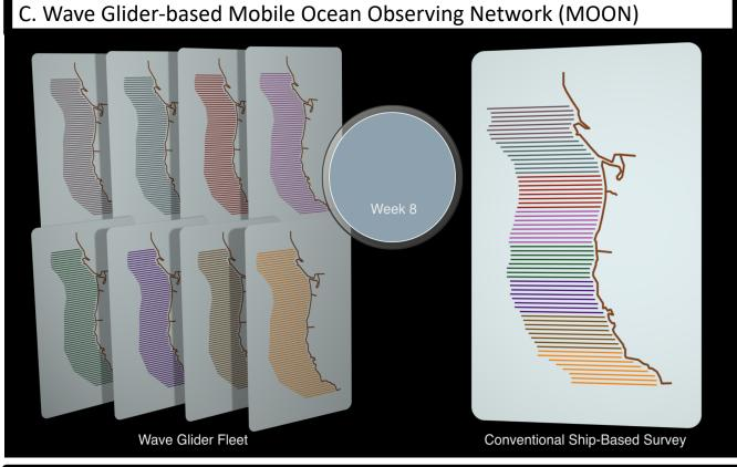
A MOON composed of a fleet of Wave Gliders can improve the synoptic nature as well as the spatial and temporal coverage of fisheries and oceanographic data collection. Our goal is to advance wave- and solar-powered vehicle technology to transform marine ecosystem and fisheries investigations into a science more consistent with ocean observing.
