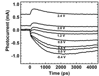
A perovskite solar cell Ultrafast photocurrent measurements
