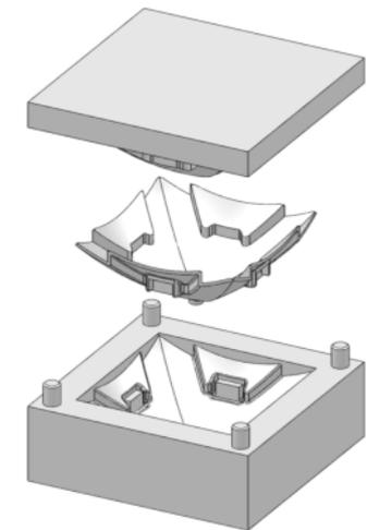
Manufacturable by single-pull injection molding
