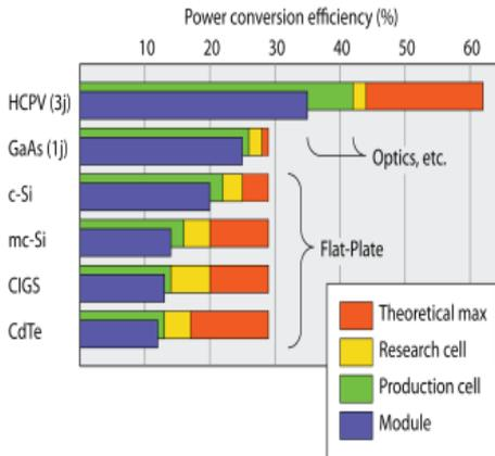
Cell Conversion Efficiency by Type and Headroom for Growth
