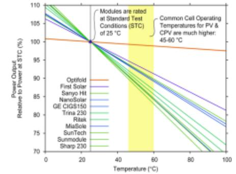
Graph illustrates temperature coefficient, In high temperatures performances decreases on all other solar, except for Optifold® with III-V
