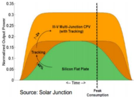
Higher Performance from higher efficiency cells and two axis tracking
