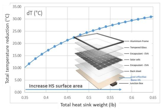
**Solution** – NanoHS reduces LCOE for solar in the field by both increase conversion efficiency (CE) and reduce solar panel peak temperature. NanoHS:
