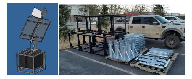
Pursuit Solar intends to initially leverage local steel fabricators and finishers to make Trackers in kit form. Approximately 1,000-3,000 ft2 of space for assembly, welding, and crating will be required. In addition, a Welder, Truck with Trailer, and Fork Truck will be needed. Mid-term vision would include bringing more of steel fabrication in-house to lower production cost. For example, a simple CNC Plasma Tube machine can be programed to make nearly all the main structural components.
