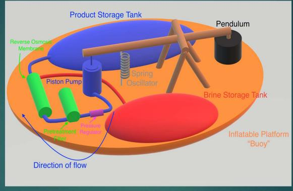
3.) As the pump reciprocates, it draws suction from the sea which it uses to pressurize the R.O. system, regulated by a check valve. As the water passes through each stage of the filtration process, contaminants, bacteria, and finally salt is removed from the seawater, making the water clean and drinkable.
