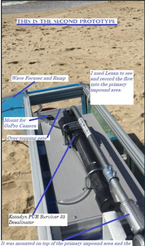
It was mounted on top of the primary impound area and th handle is connected to the buoyancy block.
