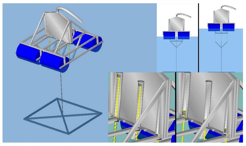
A floating platform rises and falls with each wave, while magnetic pistons are anchored to the sea floor. The magnetic pistons are free to move inside the aluminum tubes of the boiler. This motion creates heat, distilling pure water.
