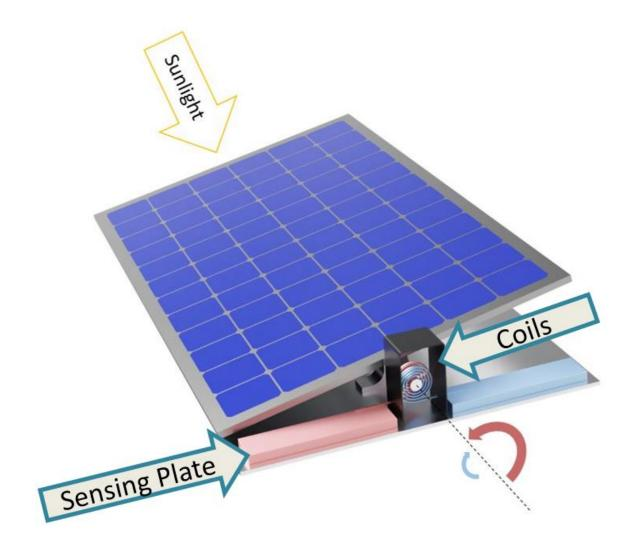
Our team is working on developing a low cost, low maintenance, and robust passive solar tracking system, which uses the temperature difference of bimetallic coils for actuation. In order to help us develop our new technology we request technical assistance in the following areas:
