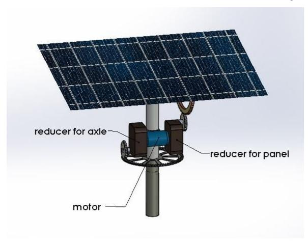
Although the regulation of these reducers can be purely mechanical based on the principles of the Antikythera mechanism
