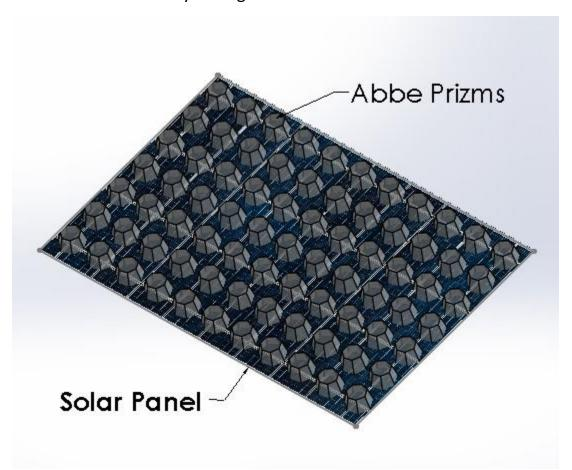
If the Abbe prisms will be too expensive, the orientation of the solar panels can be realized with a new system that is 2 times more ergonomic than the existing ones.
