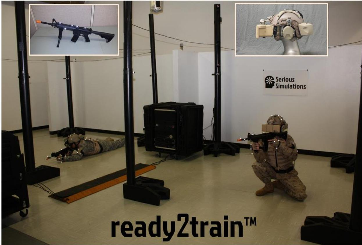
Using portable MOCAP to accommodate large or small tracking areas, individuals and teams can accomplish a variety of training or testing of equipment. Since this photo, Serious Simulations has replaced its unique wireless Head Mounted VR Display with a much improved model (see below) and we replace the spherical plastic markers with reflective tape markers wherever the 3D spheres might be cumbersome to use.
