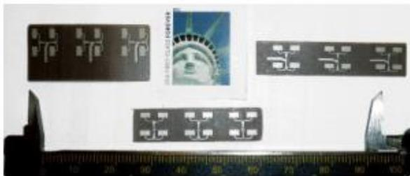
*At left is Serious Simulations' Custom steerable antenna for 60 GHz line of sight video transmission*
