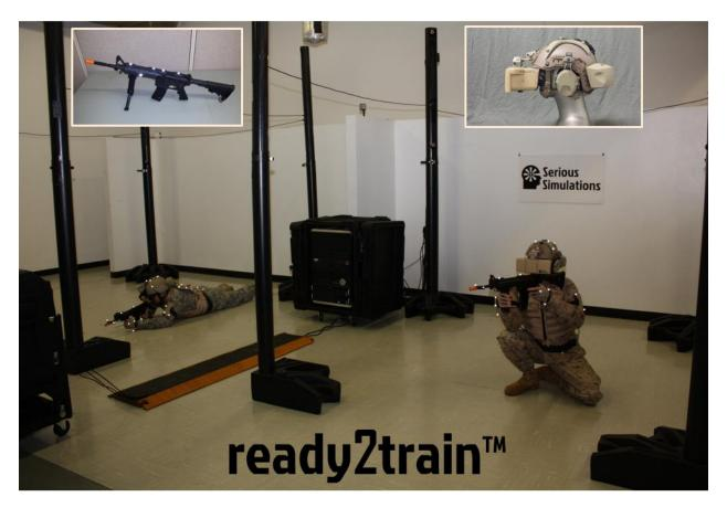
Using portable MOCAP to accommodate large or small tracking areas, individuals and teams can accomplish a variety of training or testing of equipment. Since this photo, Serious Simulations has replaced its unique wireless Head Mounted VR Display with a much improved model (see below) and we replace the spherical plastic markers with reflective tape markers wherever the 3D spheres might be cumbersome to use.
