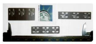
At left is Serious Simulations' Custom steerable antenna for 60 GHz line of sight video transmission
