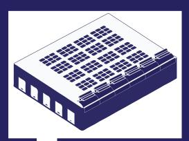
Multiple 6kW turbine modules produce about 50-200 kW on an average commercial building when installed alongside solar. Installed on the edge of the roof, where solar can't go
