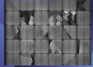
Cracks in PV Modules
