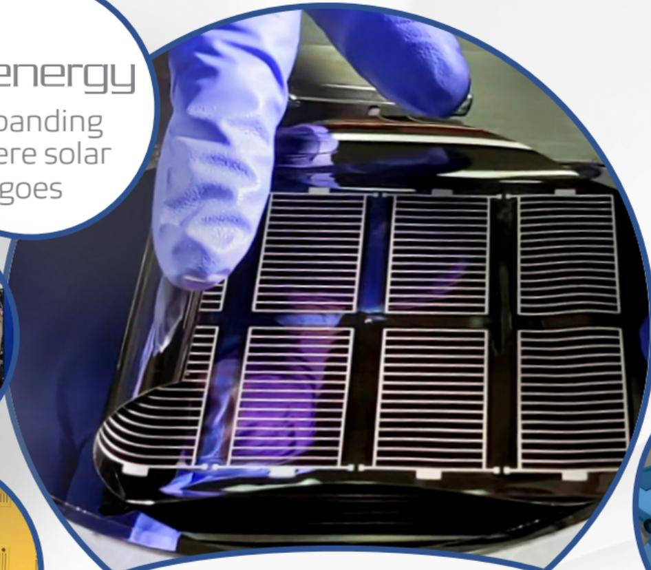
Wafer-less design with thin-film
