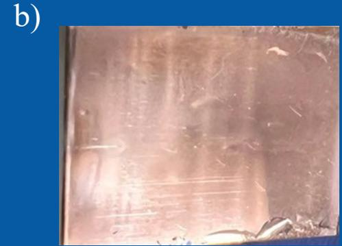
Figure 1 (a) demonstration of Cu electroplating. (b) Cu electroplated on top of Perovskite/ETL structure
