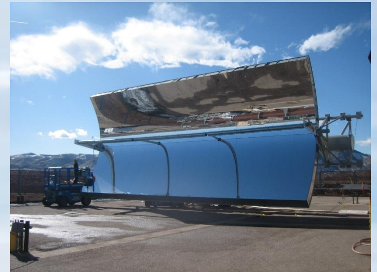
In electrical mode, Concentrating Photovoltaic (CPV) is rotated in front of the receiver (up to 44% efficient)
